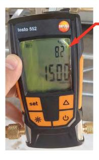
We recommend a digital Micrometer that should be connected to a bleed port under the tank, not at the vacuum pump. The micrometer pictured is capable of reading high readings approx. 75,000 microns. Most meters will not start reading until the system is less than 12,000 microns.
