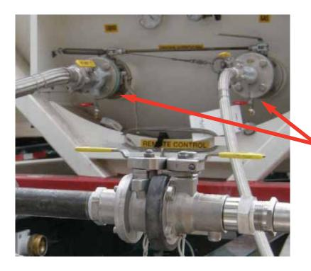
Vacuum can be pulled at these connection ports for the liquid and the vapor hoses.
