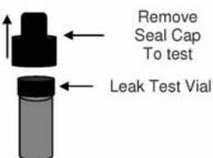
NOTE: Always remember to replace plastic seal cap after leak test is completed. Replace Test Vial when the green color is no longer visible.
