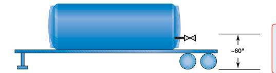
All suction piping from the hose connection to the pump should be less than 40" from grade.
