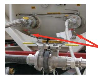
Bleed Valves for the ISO Liquid and Vapor valves.
