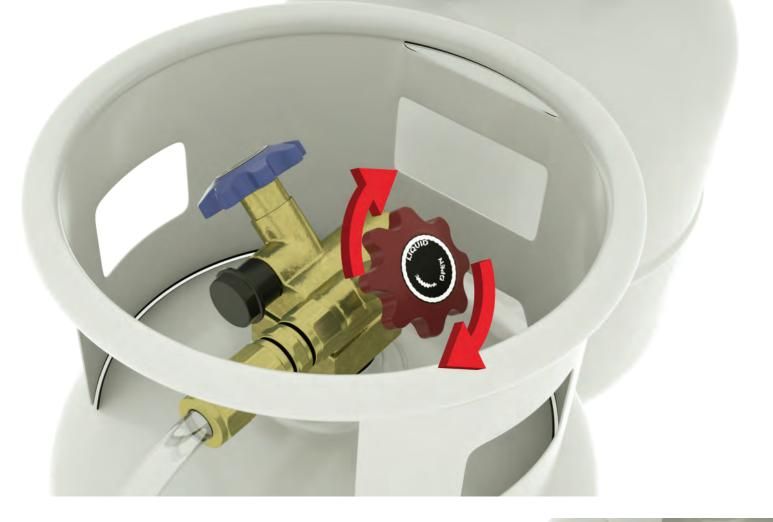
Close the liquid valve by turning handle clockwise.
