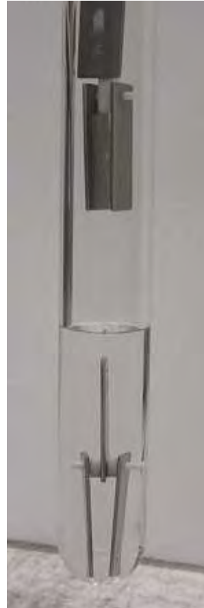
Alloy coupon set secured in HP Glass Tube w/ 80 ml of test solvent prior to placing in the water bath.
