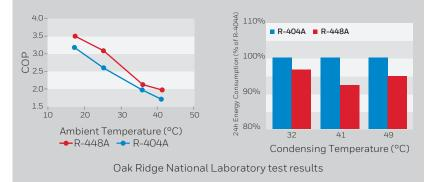
Increased operating envelope compared to other R-404A alternatives allows for a considerably lower discharge temperature when operating at low temperature conditions. This helps not only to reduce the cost of application but also helps to minimise energy consumed.
