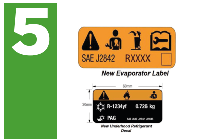
Attach new labels to identify that the refrigerant change has been made
