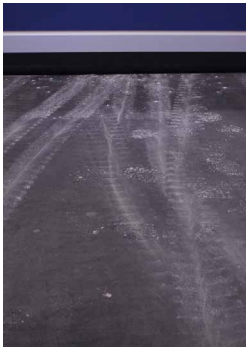
Flux powder dust scattered across the floor of a brazing area at a customer site.
