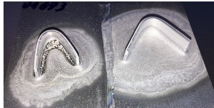
Brazing performance: left, conventional paint with high amount of organics. Right, paint formulated with XBraze concentrate
