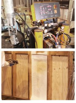
The system was sprayed on a wall assembly to test properties and evaluate the performance of Solstice LBA in the formulation.
