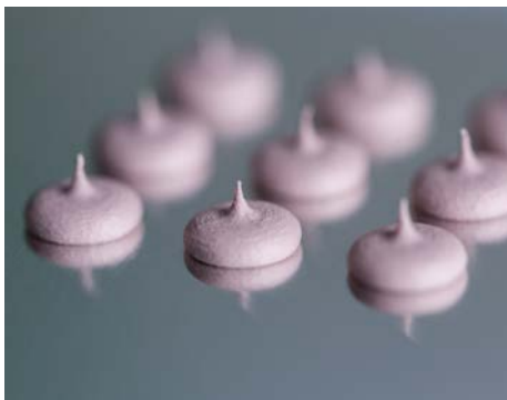
Honeywell's thermal Hybrid materials provide good surface wetting without slump after dispensing.
