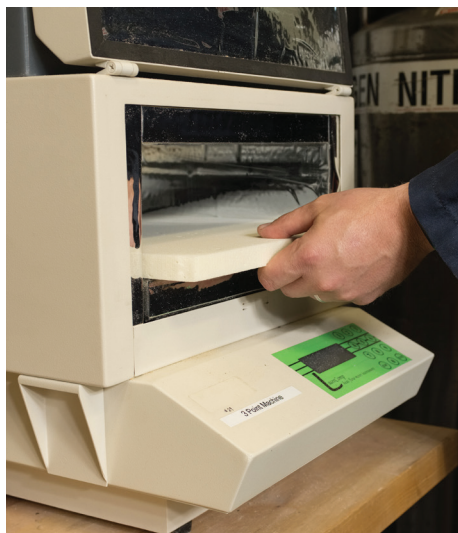
We perform extensive foam thermal conductivity testing, including testing at cryogenic temperature.
