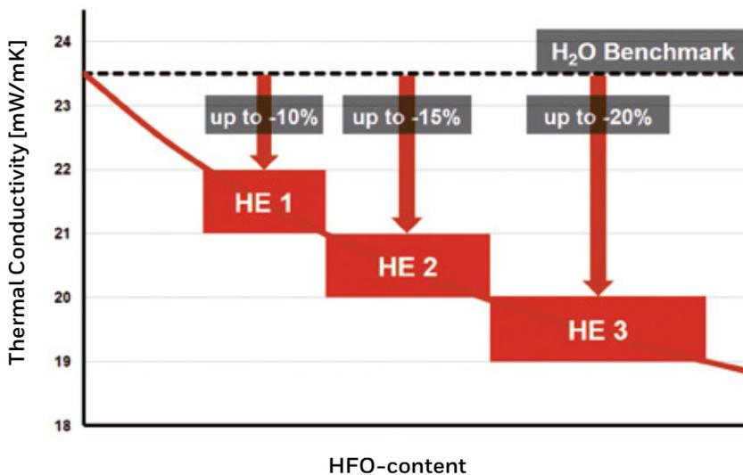
Today, BASF's Elastopor H2070 HE and Elastopor H2270 HE series are available to commercial refrigeration and water heater equipment manufacturers. They offer their customers a range of thermal performance classes from 19-22 mW/mK (HE 1, HE 2 and HE 3).
