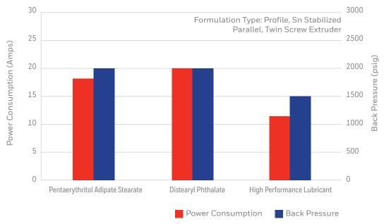
Reduced pressure, amps and temperature result in increased production capacity and operating latitude. In addition, reduced melt temperatures have been observed on full scale extrusion lines.
