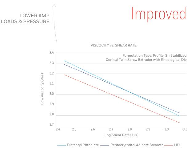
The reduction in apparent viscosity provides increased operating latitude in the extrusion process.
