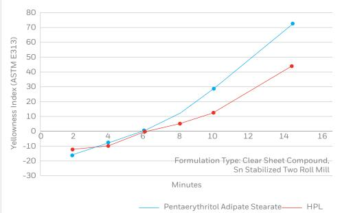
Increased color stability of High Performance Lubricant formulations suggests that there may be opportunities to reduce discoloration due to burning during the extrusion process in conjunction with increased extrusion rates.
