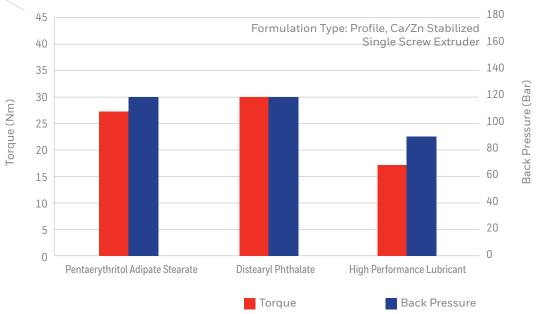
Dramatic reductions in torque and back pressure are also observed in Ca/Zn stabilized formulations as a result of the rheological effects of High Performance Lubricants.
