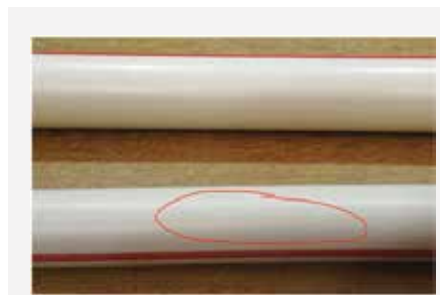
A typical example of shear burning in CPVC pipe resulting due to improper use of single ingredient lubricants and process sensitivity of CPVC resin.
